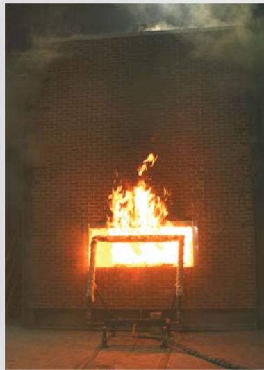
Fire emitting from the NFPA 285 test window.
