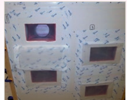
Testing real world construction joints at the Owens Corning lab allows us to determine the impact of sealing the most important air leaks.
